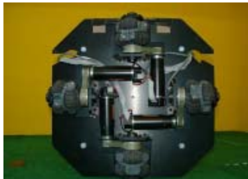
Fig. 2 Omnidirectional Mobile mechanism
